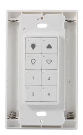
Short press: Sends "ON" instruction to lights that are bound to this switch and also controls its local Relay to ON position.
