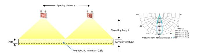
NFPA 101 requires 1.0 foot-candle average and 0.1 foot-candle minimum with a 40:1 maximum/minimum ratio. The corridor used is 100feet long, 10 feet ceiling with a 6 feet wide walkway and 6&3 feet path of egress for calculation. The reflectance are 80% ceiling, 50% walls and 20% floors. The fixture mounting height is 7.5 feet /10ft.
