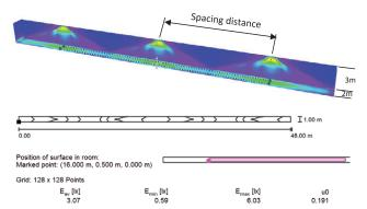
Compliant EUROPE standard EN1838 Illuminance requirement: Escape route up to 2 m wide,1 lx on the central axis and 0.5 lx at 50% of the width.
