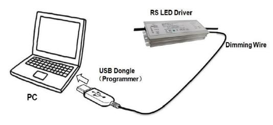
The programmable driver can be programmed by using special PC software and the programmer module.
