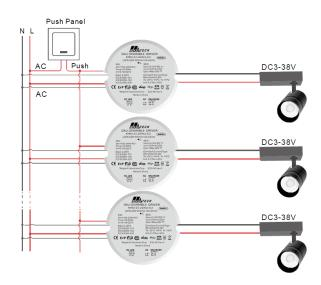
Remark: Only use open push button without indicator light. Maximum cable length between each unit: 20 meters.
