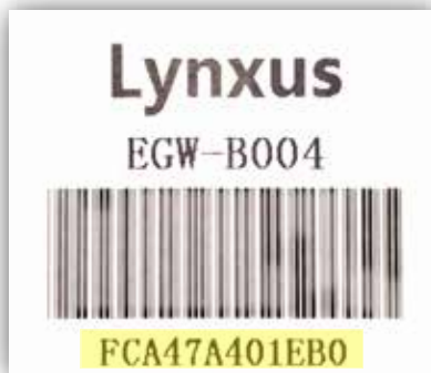
Figure 1: Example serial number sticker located on the back of a gateway device. The serial number is highlighted in yellow. In this instance, for a standalone gateway configuration, the Wi-Fi network the user should connect to is: “LYNXUS_ZGW-401EB0”. Additionally, The associated gateway password in this case would be: “7A401EB0”
