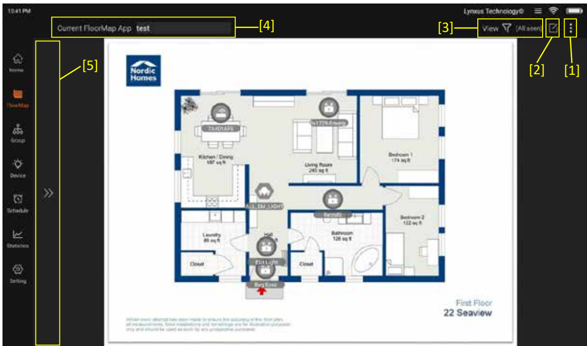
Figure 5: LynxEM Floor Map Screen. This is the layout of the Floor Maps page within the LynxEM application. Functions mentioned above are numbered in yellow.
