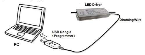
The programmable driver can be programmed by using special PC software and the programmer module.
