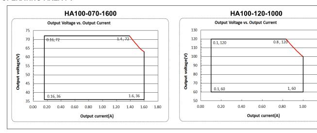
Notes: X=N is suitable for the right area of the dotted line; X=P is suitable for the solid line contain area.
