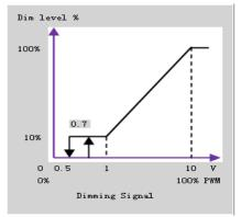
Click ON "☑"to activate dimming signal configuration, the dimming signal can be analog or PWM signal, here to set the value of the high level of these two signals, the setting can be:
